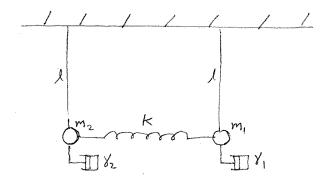
We could add sinusoidally varying driving forces, but we'll stick with the transient (homogeneous problem) case for now. To get you started, here is the force equation for mass 1:
